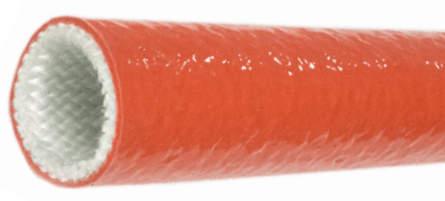
(260°C) AND WILL WITHSTAND A MOLTEN SPLASH AT 2200°F (1200°C). MADE OF KNITTED FIBERGLASS YARNS IN A FLEXIBLE SUBSTRATE, THIS PRODUCT IS THEN COATED WITH A HIGH GRADE SILICONE RUBBER.
